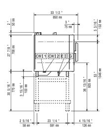
Cold Water inlet 1 (cleaning) CWII CWI2 = Cold Water Inlet 2 (steam generator)
